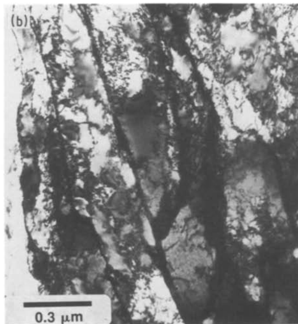
Figure 5 Pure copper specimen tested at 400°C. (a) Scanning electron micrograph of the fracture surface; (b) transmission electron micrograph of dislocation substructure immediately adjacent to the fracture surface. By comparison with the room-temperature pure copper sample (Figs 2b, 3b) the microvoids and dislocation cells appear more well developed at 400°C, although the absolute cell and microvoid sizes appear unchanged.
